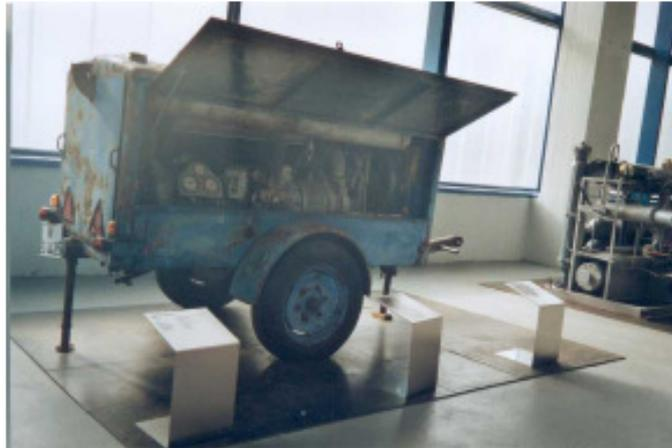
The compressor was built at the last company formation, *Junkers – Maschinen –und Metallbau* Munich-Allach, in 1958. It was used in road construction. It is a mobile free piston compressor with a two-cylinders diesel engine.
