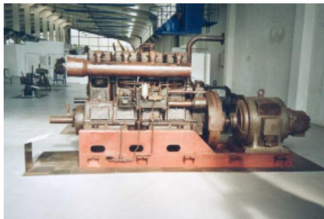
This in-line diesel engine with 4 cylinders was produced at the Junkers factory *Gesellschaft für Dieselkraftmaschinen* in Chemnitz around 1930. The generator was delivered by *Fa. Keiser* from Berlin. The engine and the generator are connected to one another by means of an elastic connecting link. This engine version is a ship engine. It was started by use of air compression in the cylinders. The engine you see was used at Dessau waterworks as an emergency generator.
