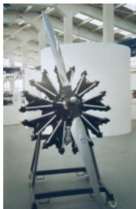
This nine-cylinder radial engine was normally used in Ju 52. This 660-HP engine with a weight of 430 kg had some advantages over Junkers diesel engines. As a petrol engine with an air cooling it was, in addition, equipped with an oil cooler. Every cylinder had got two sparking plugs with an ignition system for reliable ignition.
