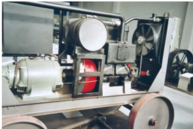
This is a two cylinders in-line diesel engine, built in Chemnitz in 1935. Engine and generator are installed on a chassis frame and served as electricity supplier in rural areas. The efficiency of the generator is 19 KVA. The starting occurs electrically.
