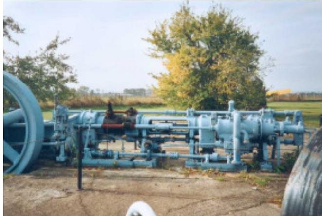
It is the first oil engine built according to the principle of dual pistons. It was used for experiments with various lubricants, experiments on fuel injection system, and for search of ways of increasing capacity. The second cylinder was installed later. This version, known as tandem engine, had a capacity of 2×100 HP.
