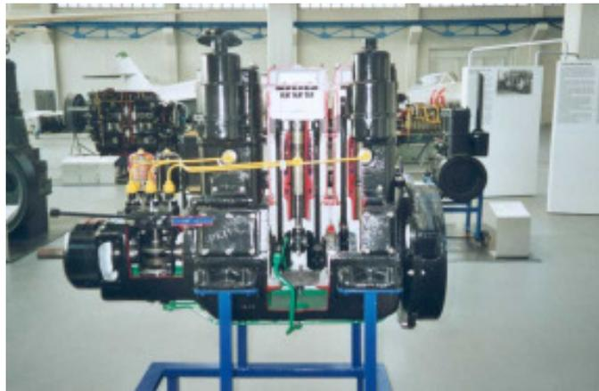
This diesel in-line engine with three cylinders was built in 1925 and installed in a truck. It is fitted out with a flywheel and a torsional vibration damper to improve imbalance. The engine was started with a battery. Cylinders and some other parts of the engine are shown in section.
