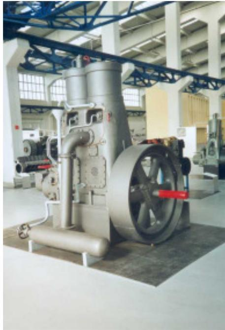
*Junkers-Motorenbau GmbH* was the producer of this two-cylinders in-line diesel engine of 1930. It was produced for industry and ship use. The flywheel is suited also for flat belt connection. The compressed air is annealed by means of a cylinder with compressed air container
