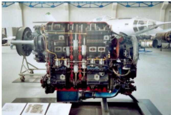
This is an opposed piston aircraft engine with an efficiency of 680 HP. It was manufactured at *Junkers-Flugzeug und Motorenwerken Dessau* and used in the military planes Ju 86 and BV 138. It was built in 1938.
