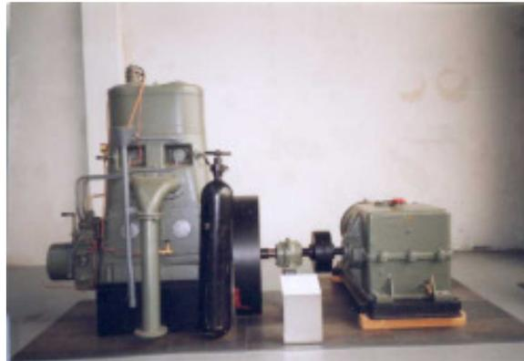
This set was produced at *Junkers-Motorenbau Dessau* around 1930. The engine was started with compressed air from the compressed air containers. There is a flexible spike coupling between the engine and gearbox. The centrifugal pump is directly and fixedly added on the gearbox. The engine was at the waterworks Dessau.
