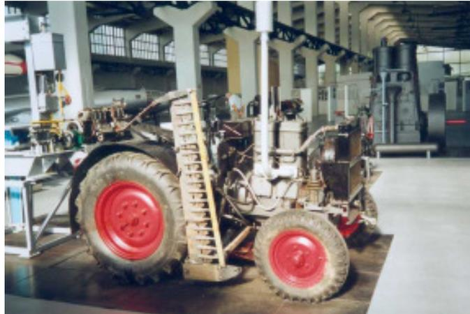
It was built as a tractor with a modified Junkers engine at *VEB IFA, Ingenieurbetrieb Hohenstein-Ernstthal*, after the Second World War. The starting occurs electrically or by means of a crank. The tractor is still in working condition.
