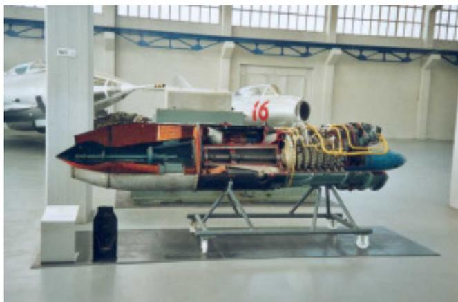
The power unit was already developed in 1940/41. The B version was mass-produced with an eight-stepped axial compressor. It ran on kerosene and had an efficiency of 900 kp.
