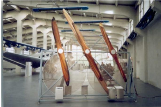
The shown airscrews are made of wood. These are fixed pitch propellers with predetermined angle of blades. Variable pitch propellers with wooden airscrews were used later, too. The airscrews are made of tropical timber, the sheets of wood were glued together in layers. *Heine* company from Berlin supplied Junkers workshops with wood plates. Metal airscrews (aluminium) were also developed and manufactured by Junkers.
