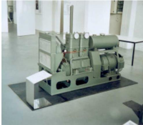
Till the beginning of 1960s engines with domed pistons from the HK-series were produced according to Junkers' patent, almost unchanged, at *VEB Dieselkraftmaschinenwerk Karl-Marx- Stadt*, the succession company of *Junkers Dieselkraftmaschinen GmbH Chemnitz*. This diesel engine was produced in 1957. It had two cylinders arranged in line. The engine was connected to FIMAG generator by means of an elastic connecting link. The engine was started electrically.
